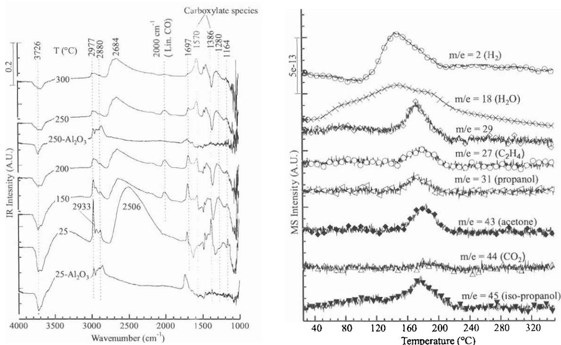
Figure 8. IR and MS analysis during TPD of iso-propanol over Rh/Al<sub>2</sub>O<sub>3</sub>
