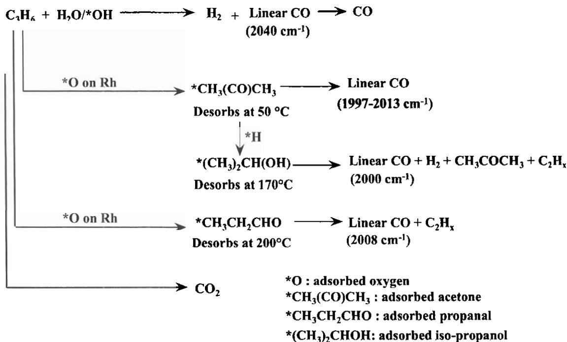
Figure 9. Reaction pathway for propylene partial oxidation over Rh/Al<sub>2</sub>O<sub>3</sub>.
