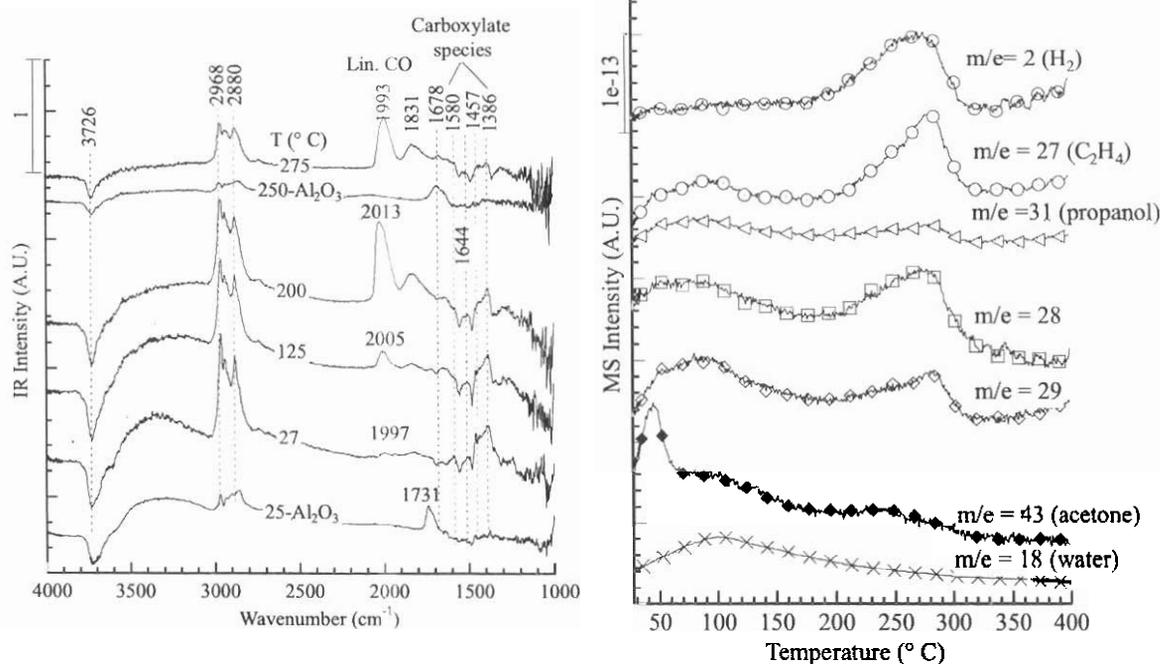
Figure 7. IR and MS analysis during TPD of acetone over Rh/ $\text{Al}_2\text{O}_3$ .
