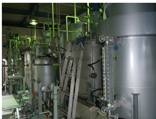
Figure 2: Battery of hydrolyzing reactors whose composition and activity is being precisely tailored according to the biochemical composition and level of disintegration of the substrate.
