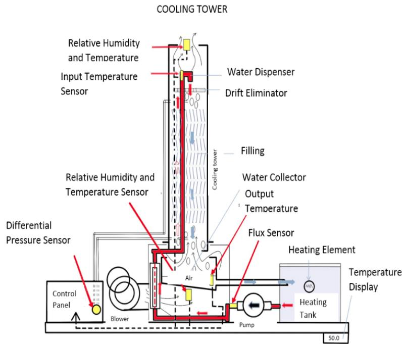
Figure 9. Schematic diagram of the cooling tower
