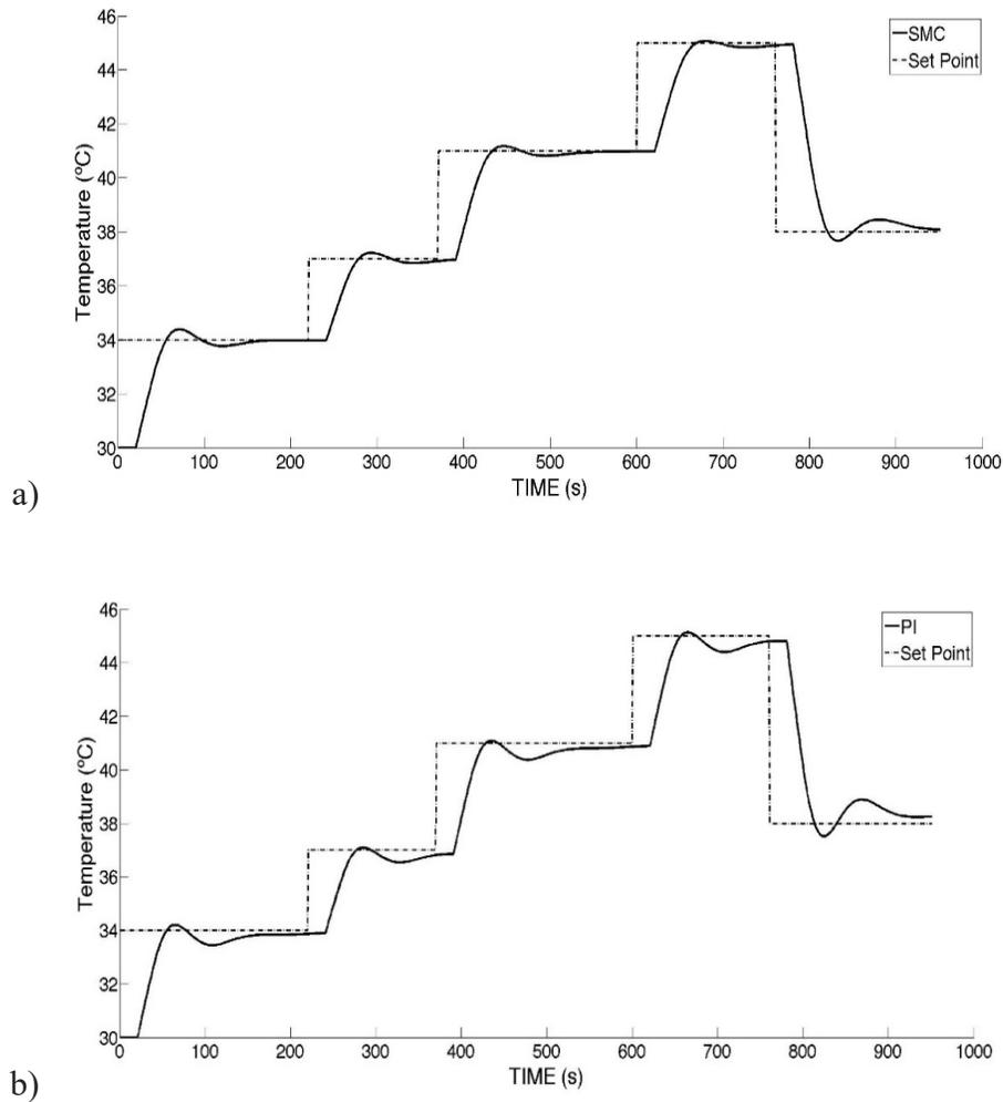
Figure 10. Simulation responses for set point changes
