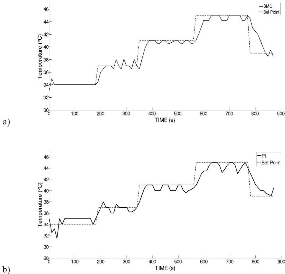
**Figure 11.** Experimental results for set point changes
