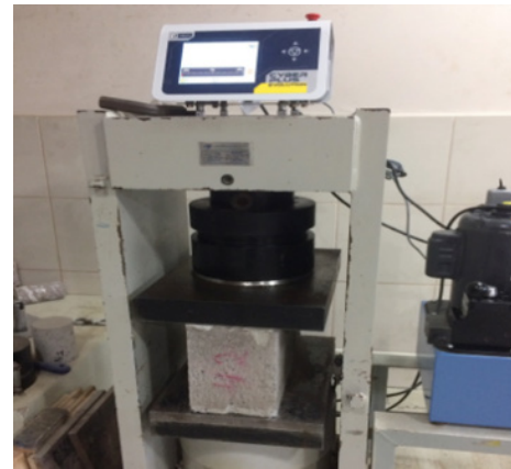
Figure 7. Prototype block compression test.
