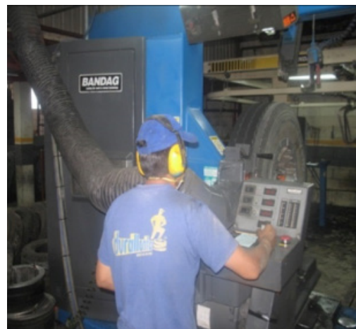
Figure 1. Blade machine for the scraping process.
