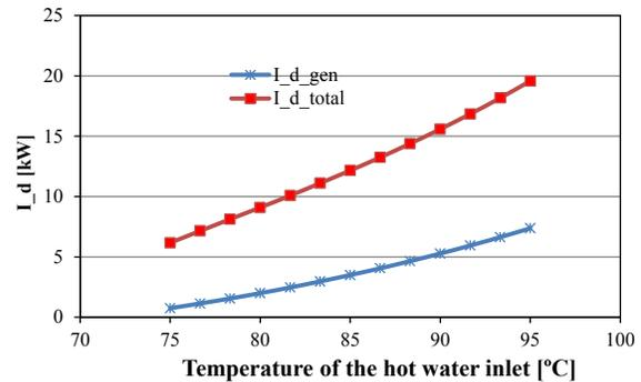
Figure 5. Change in the destruction of total Exergy and of the generator as a function of the inlet temperature of the hot water to the generator.
