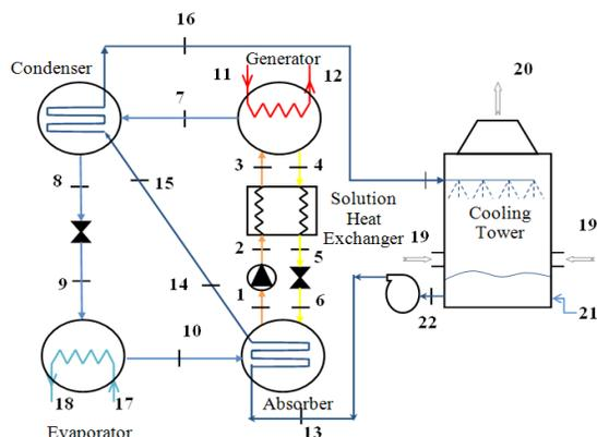
Figure 1. Single Stage Absorption Cycle.
