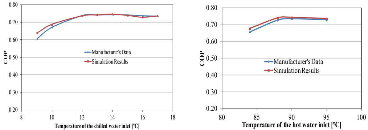
Figure 3. a) Comparison of the COP between the data supplied by the manufacturer and those obtained by the simulation, for a hot water temperature of 95°C. b) Comparison of the COP between the data supplied by the manufacturer and those obtained by the simulation, for a chilled water temperature of 7°C.
